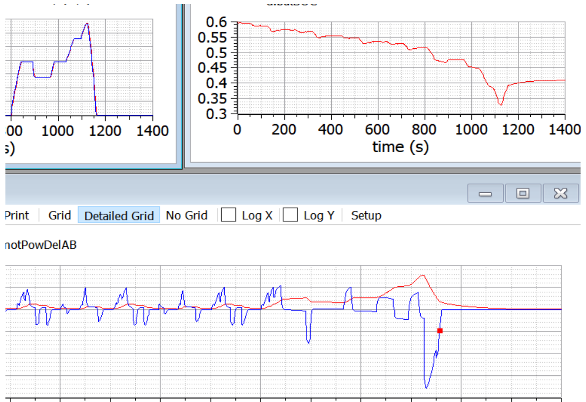
Figure 49 Some plots obtained when simulating the model in figure 45 (EHPTexamples.PSD.PSecu1), controlled with the ECU shown in figure 48 (ECU1) subject to NEDC cycle.
